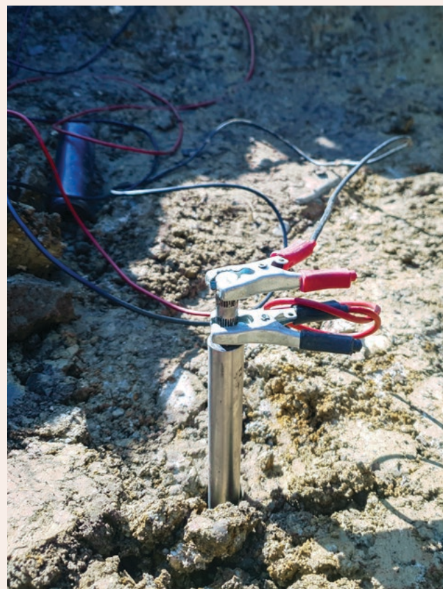
Figure 21: Example of an earthing device with a POS K Rf earth rod
