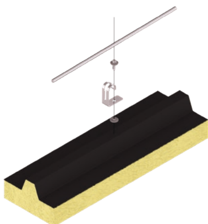
Figure 6: Installation of a suitable load-bearing element on a trapezoidal roofing.
