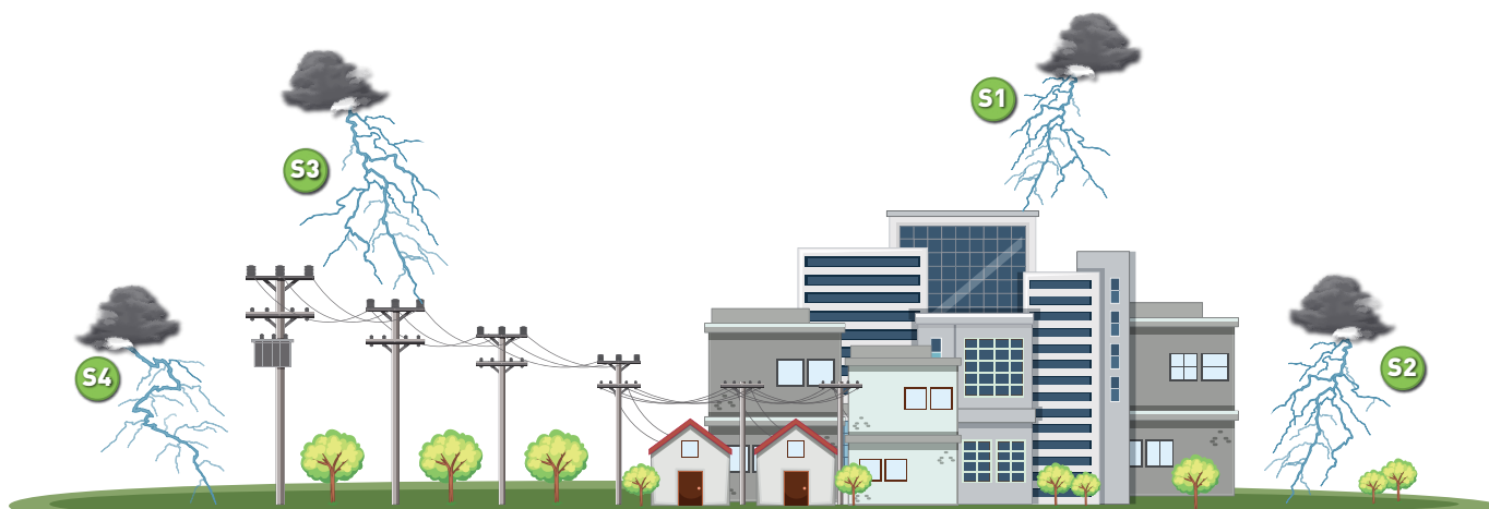
Figure 1: Source of damage according to lightning strike points
